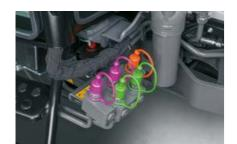
Up to four hydraulic connections and a free-flow return are available at the front
