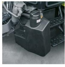
The 105 I diesel tank and the 10 I urea tank provide enough range for long working days
