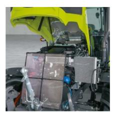
You can slide out radiator and remove the radiator screen in no time for inspection and cleaning
