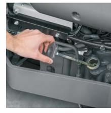
The oil level can be checked and topped up on the right-hand side of the ELIOS 300 when the bonnet is closed
