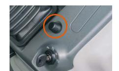
Use the rotary switch beside the steering column to navigate easily through the menu
