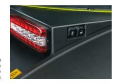
Draught control, lowering speed and lift height limiter can be operated from the right-hand console
