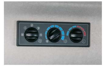
The controls for the air conditioning are within easy reach on the right-hand side of the cab roof liner
