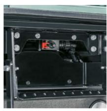
The battery isolating switch is conveniently located on the left access step
