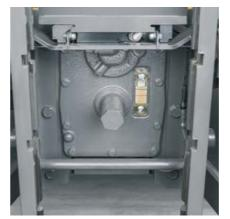
You can check the transmission and hydraulic oil level in a sight glass next to the rear PTO stub
