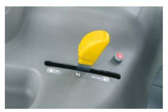
The electrohydraulic PTO engagement controls the start-up smoothly to suit the attached implement and protects the mechanical components
