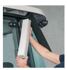
The cab air filter is easy to access from outside for cleaning and keeps the air in the cab fresh at all
