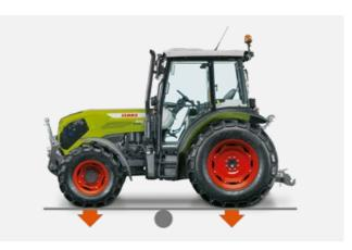
CLAAS supplies optional factory-fitted Trelleborg turf tyres (sizes: 600/55-26.5 rear and 00/55-22.5 front) to enable the ELIOS to be driven over sensitive grass cover or wet subsoil in parks and on sports fields without damaging the precious turf – all year round.
